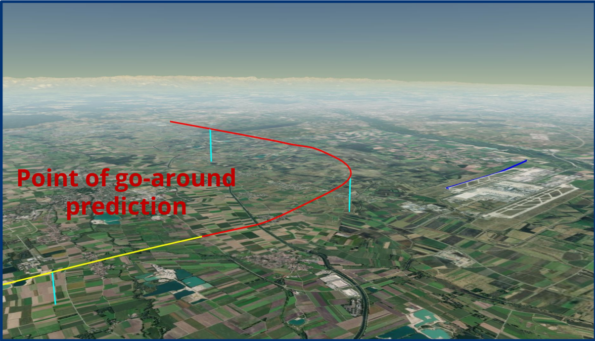
Trajectories of simulated aircraft with prediction
