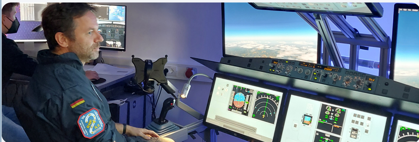
A321 cockpit simulator based on X-Plane 11 software
